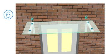
K Marry all holes in the glass with holes in the brackets. If any holes don't align, you may need to loosen the odd fixing in the bracket/wall and pack where required and tighten back up.
