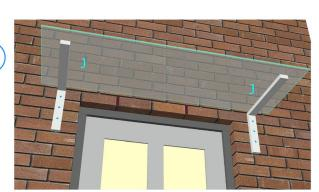
J Remove pre-assembled fixings from the brackets. Sit glass onto the brackets.
