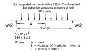
Deflection calculation of Heavy Duty Self Supporting Glazing Bar Fail point beyond a deflection of 35mm under maximum
